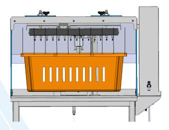
After few test on the machine, simulating a 'standard' condition, (18ml spray; 25ml gel; 100 chicks) the machine complete a full cycle of administration in about 8-10 seconds (including the operation of insert and take out the box).
