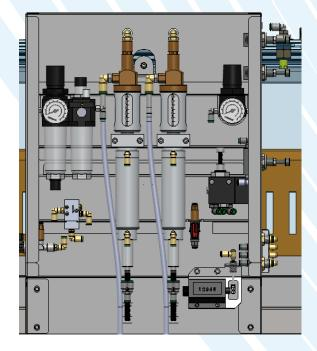
The device Is equipped with 4 nozzle adjustable in 4 direction to fit with every box, and a gel bar with 14 needle that moves trough the cabin to cover all the chick box.
