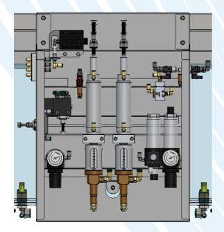
The device Is equipped with 4 nozzles (Dispensing the 1st vaccine) adjustable in x-y direction and 2 nozzles (Dispensing the 2nd vaccine) adjustable in y direction to fit with every box dimension. The machine is also equipped with an adjustable piston to block the box until the end of dispensing
