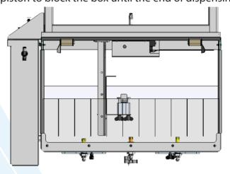
After few test on the machine, simulating a 'standard' condition, (18ml 1st spray; 18ml 2nd spray; 100chicks) the machine complete a full cycle of administration in about 8-10 seconds (including the operation of insert and take out the box).
