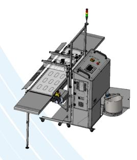
The machine thanks to the PLC and the photocell installed on is able to adapt to every hatchery conveyor system. In case your hatchery do not have a conveyor system the machine can be supplied with his own conveyor. This conveyor can be also disassembled in case you have your own conveyor system.
